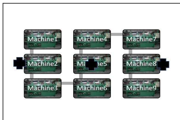
Figure 2. The pattern of noise monitoring in the production process; ■ = sound level meter point for monitoring the noise level.
