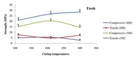
Figure 7. Effect of curing temperatures on fresh tailings strength after stabilization.
