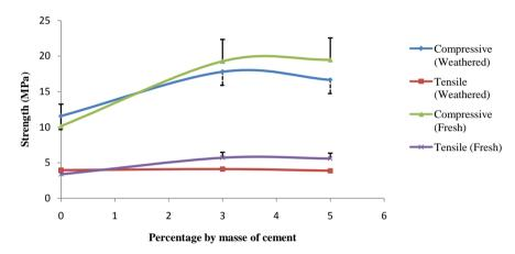
**Figure 5.** Effect of percentage by mass of cement on tailings strength after stabilization.
