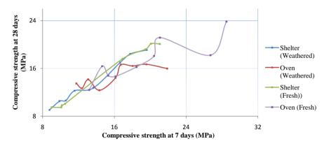
Figure 9. Effect of the time on tailings strength after stabilization.
