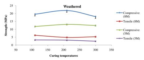
**Figure 8.** Effect of curing temperatures on weathered tailings strength after stabilization.
