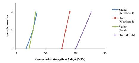
Figure 11. Effect of the drying method on tailings strength after stabilization.
