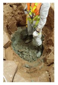
Figure 2. Ongoing digging of a sampling pit.
