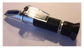
Figure 1. Hand-held optical refractometer.
