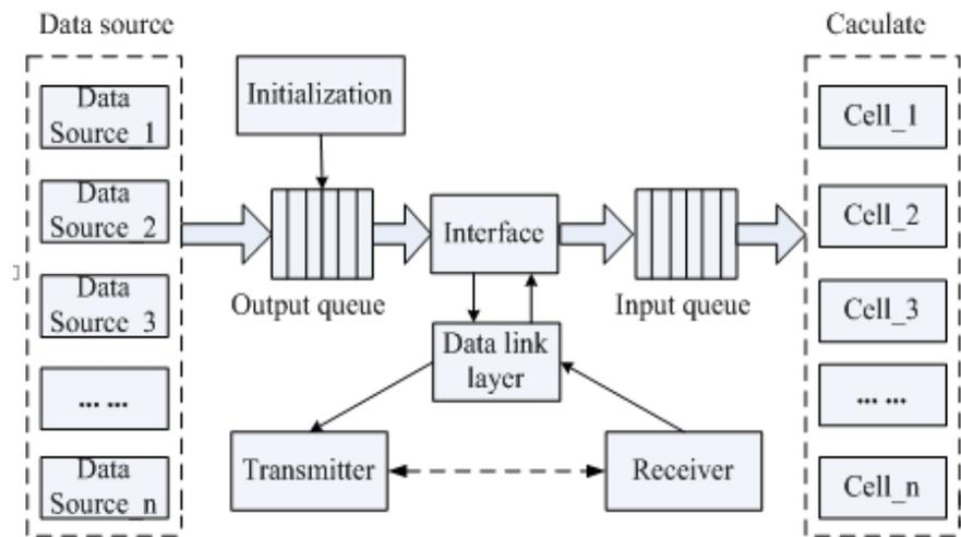
**Figure 2.** Merging unit model of smart substation.
