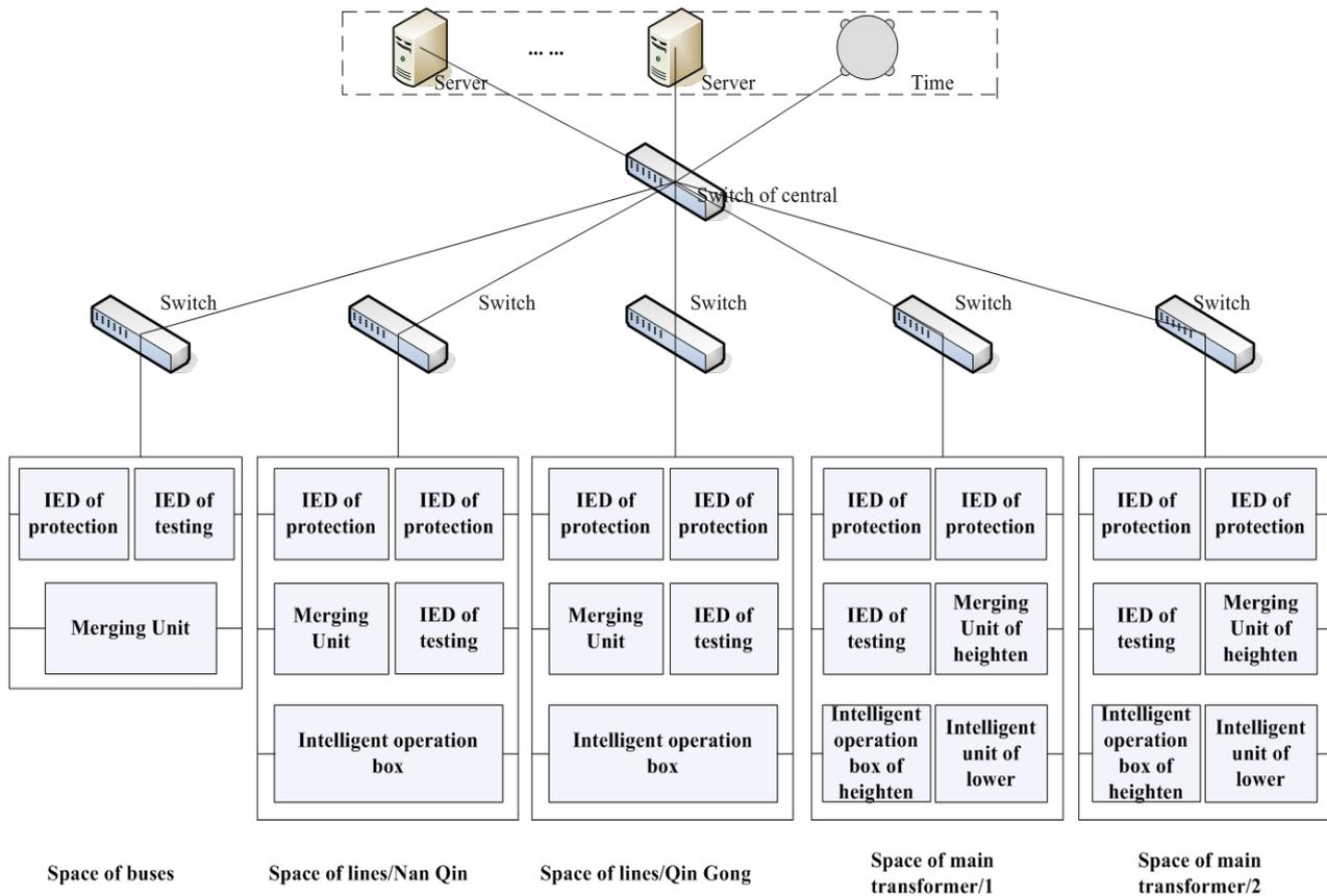
Figure 4. Topology of 110 kV communication network.
