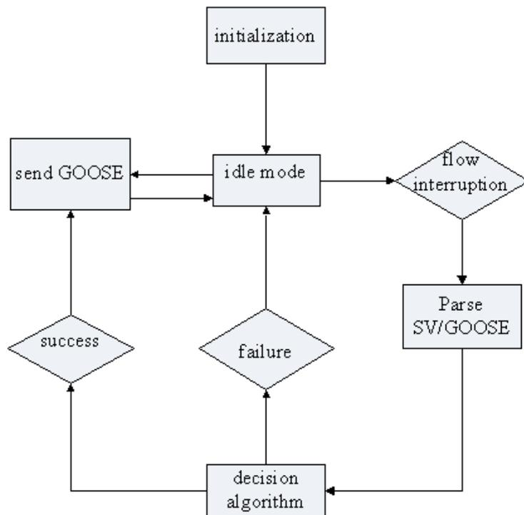
**Figure 3.** State transition of the application layer.
