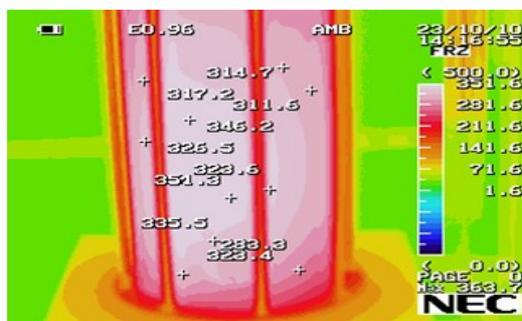
**Figure 4. Thermal infrared imager image of quartz reactor wall at fluid gas 4 m<sup>3</sup>/h (quartz sand 21.3 g and operation power 10 kW).**
