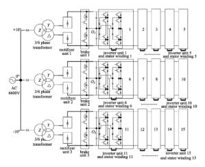
Figure 1. The topology of the high power fifteen-phase propulsion converter.
