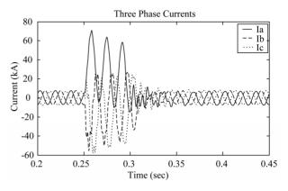
Figure 7. Three phase current waveforms during 3LG fault before the UPFC.
