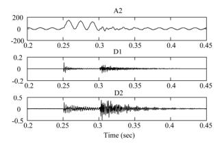
Figure 4. Approx. and details of phase A current during 3LG fault before SSSC.
