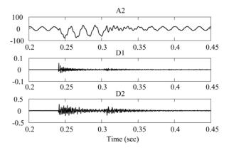
Figure 6. Approx. and details of phase A current during 3LG fault after SSSC.
