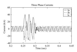
Figure 9. Three phase current waveforms during 3 LG fault after the UPFC.
