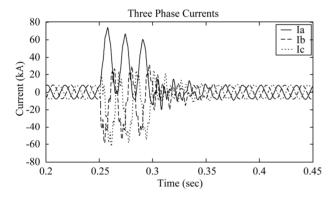
Figure 3. Three phase current waveforms during 3LG fault before the SSSC.
