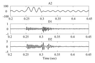
Figure 10. Approx. and details of phase A current during 3LG fault after UPFC.
