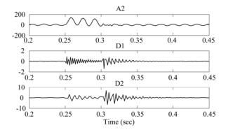
Figure 8. Approx. and details of phase A current during 3LG fault before UPFC.
