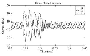
Figure 5. Three phase current waveforms during 3LG fault after the SSSC.
