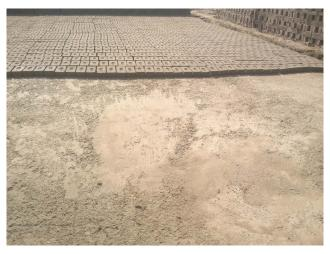
Figure 4. Clay bricks are being placed on ground for drying.
