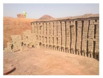
Figure 5. Sun dried clay bricks are being placed for firing in kiln.
