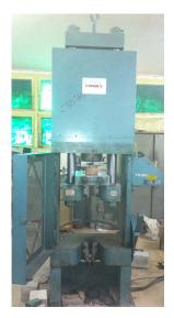
Figure 7. A baked clay brick specimen is being tested for compressive strength in Universal Testing Machine.
