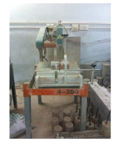
Figure 6. A baked clay brick is being cut into two halves using cutter machine.
