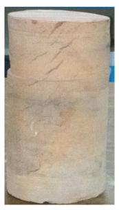
Figure 3. A baked clay cylinder core of 150 mm diameter and 300 mm height.
