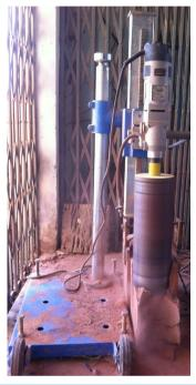
Figure 2. A baked clay cylinder is being cut with core cutter machine.
