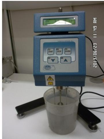
Figure 6. Rotary viscometer device.
