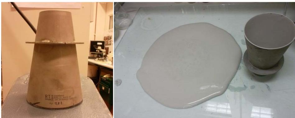
Figure 8. Left figure shows the mini slump cone and right figure shows the final spread of a grout in the mini slump test.
