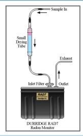
Figure 2. Schematic diagram for the Radon measurement in indoor air.
