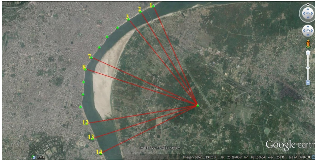
Figure 3. Bifurcation of cross-sections at Varanasi Bend of River Ganga.
