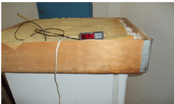
Figure 14. Small-scale model of the heating sand floor photographs.
