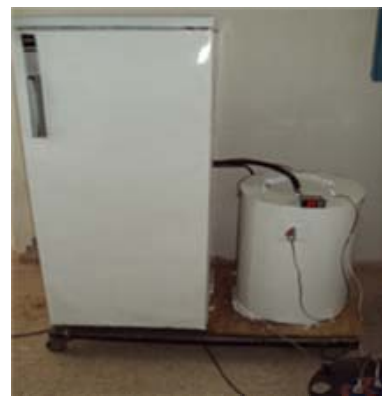
Figure 11. Coupling of the refrigerator to a water-heater photograph.
