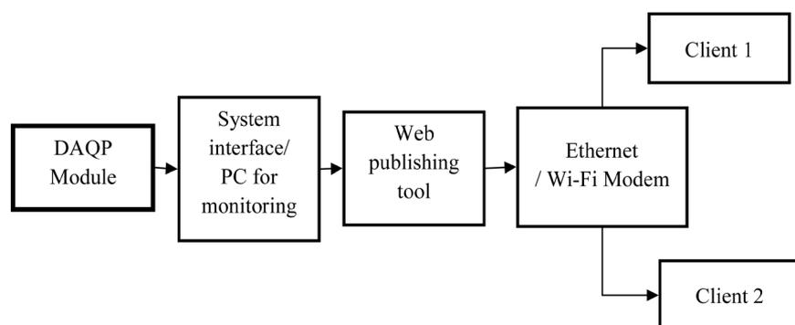
**Figure 3.** Network control module.
