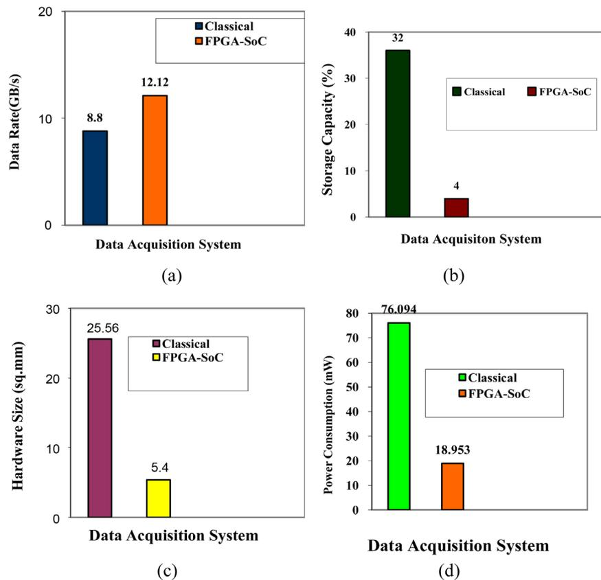
**Figure 12.** Performance analysis of proposed FPGA-SoC based DAQ system (a) Data rate speed (b) Storage capacity (c) Hardware size (d) Power consumption.
