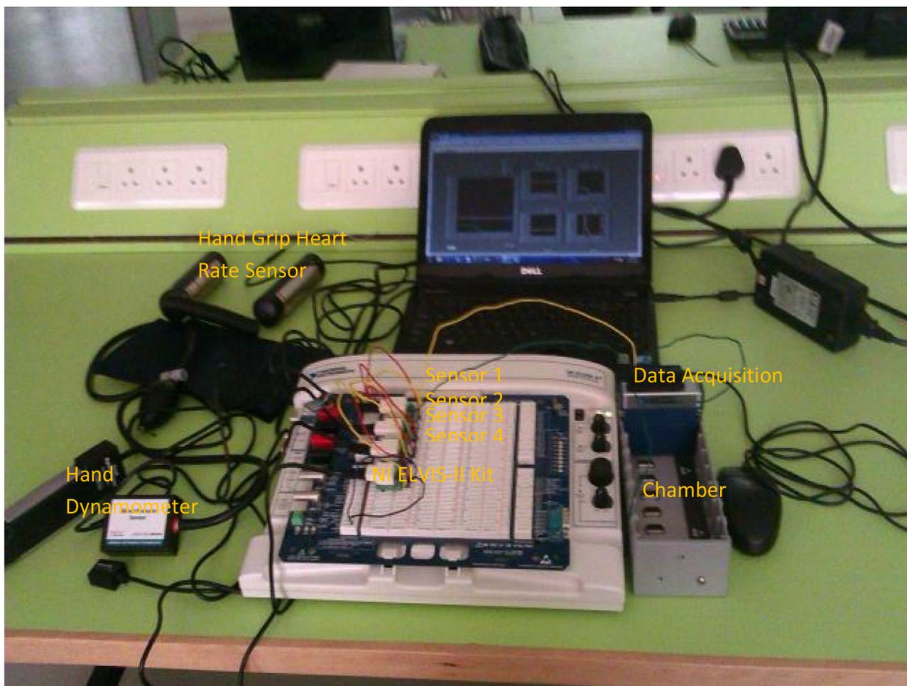
**Figure 4.** Experimental setup of multichannel DAQP.
