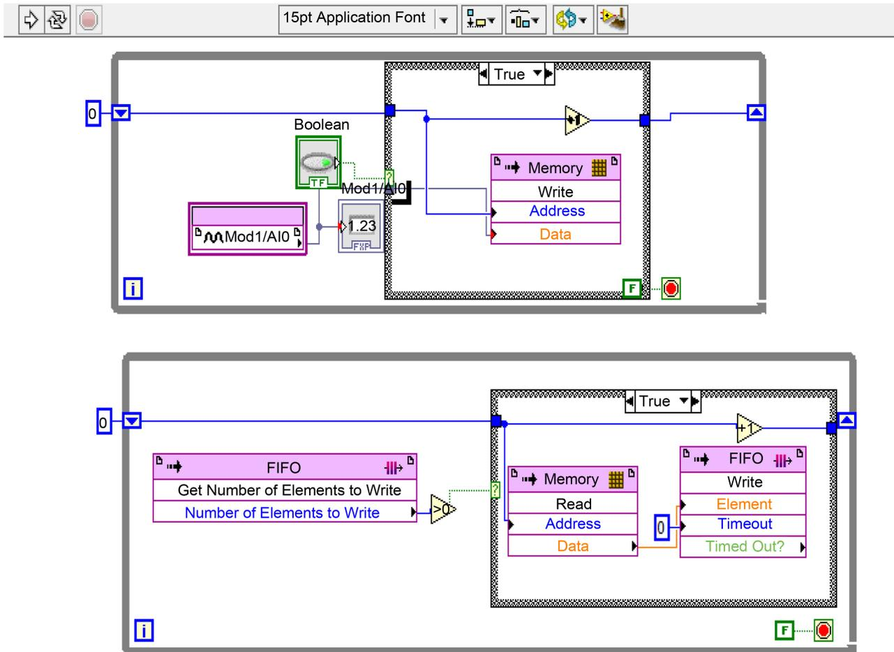
Figure 9. Design of FPGA target.vi for multichannel DAQP using LabVIEW G-code.
