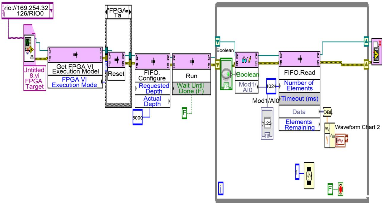
Figure 10. LabVIEW G-code for FPGA host.vi.
