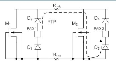
Figure 5. Main discharge path for a PTP mode.
