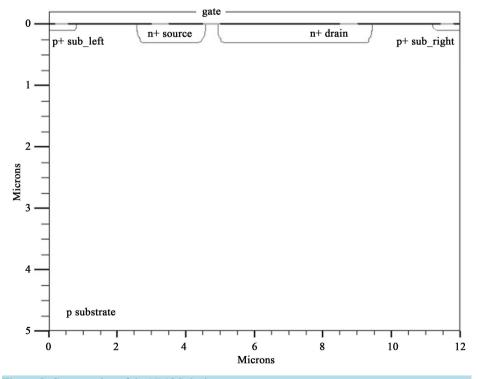
Figure 2. Cross section of the NMOS device.
