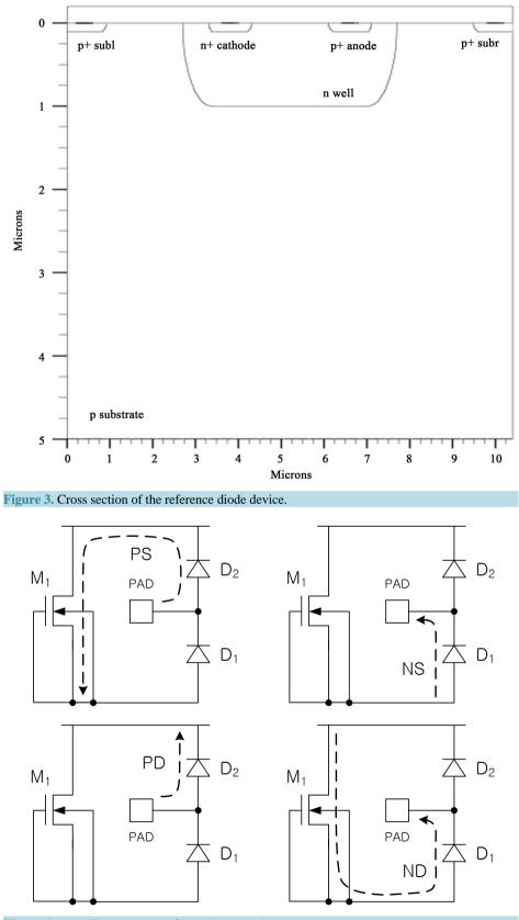
Figure 4. Main discharge paths for each test mode.
