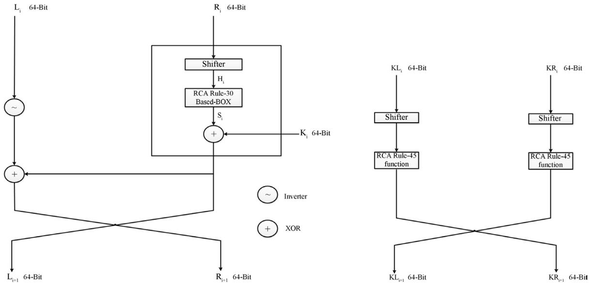
**Figure 1.** Encryptions/decryption round function and key scheduling of KAMAR.
