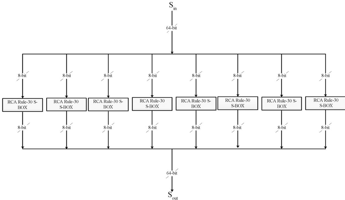
**Figure 2.** Internal structure of RCA rule-30 based S-BOX.
