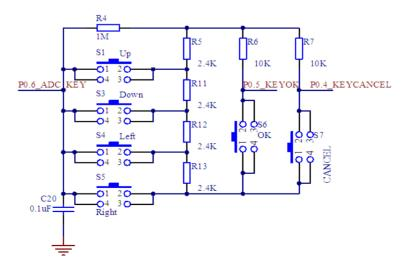
Figure 3. Switch control circuit.
