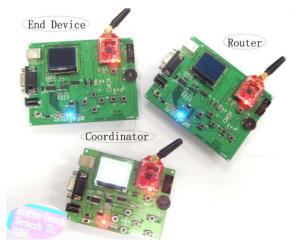
Figure 8. Wireless light control networking.
