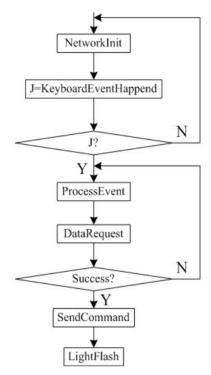
Figure 7. Key light control algorithm.
