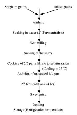
Figure 1. Flow diagram for the traditional processing of kunu-zaki from composite grains.
