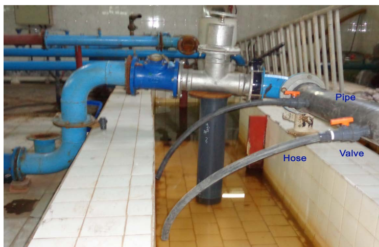
Figure 3. Laboratory calibration for gated pipe line.
