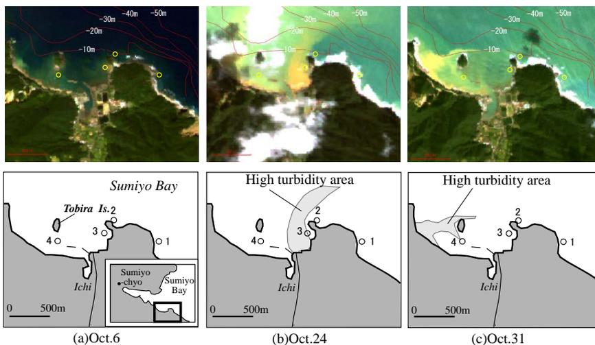
**Figure 5.** Comparison of ALOS AVNIR-2 images with the bathymetric line around Tobira Island before and after heavy rain in 2010.
