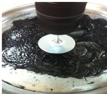
**Figure 5.** Dispersing process of nonfunctionalized CNTs in epoxy resin.
