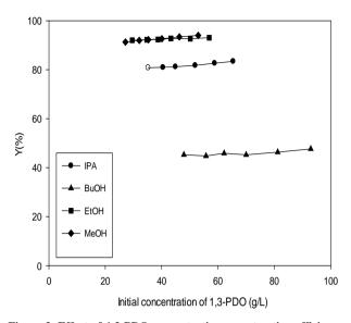
Figure 3. Effect of 1,3-PDO concentration on extraction efficiency in an aqueous two-phase systems composed of  $Alcohols/K_2HPO_4$ .
