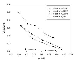
Figure 2. Phase diagram of alcohols/salt aqueous two-phase systems.
