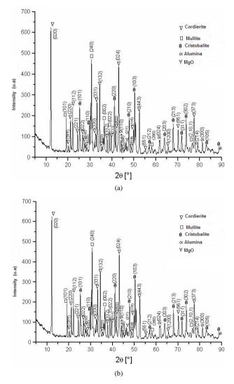
Figure 1. Patterns of X-ray Diffractions: (a) mix I, (b) mix II burned.
