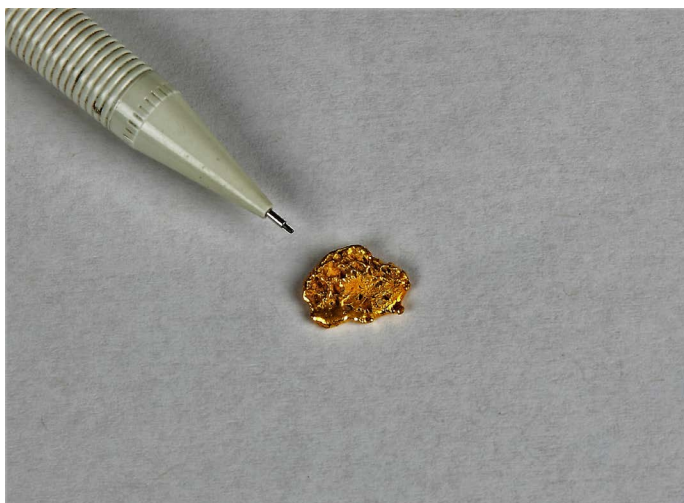
Figure 6. Anthropogenic gold nugget from Puerto Maldonado, Perú showing sponge-like texture resulting from burning (Spanish, refogado ) the mercury-gold amalgam to volatilize the mercury.
