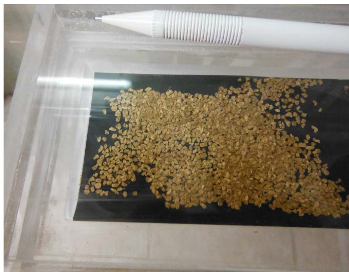
Figure 7. Byproduct gold concentrate at Pomza Export office showing flattened grains.
