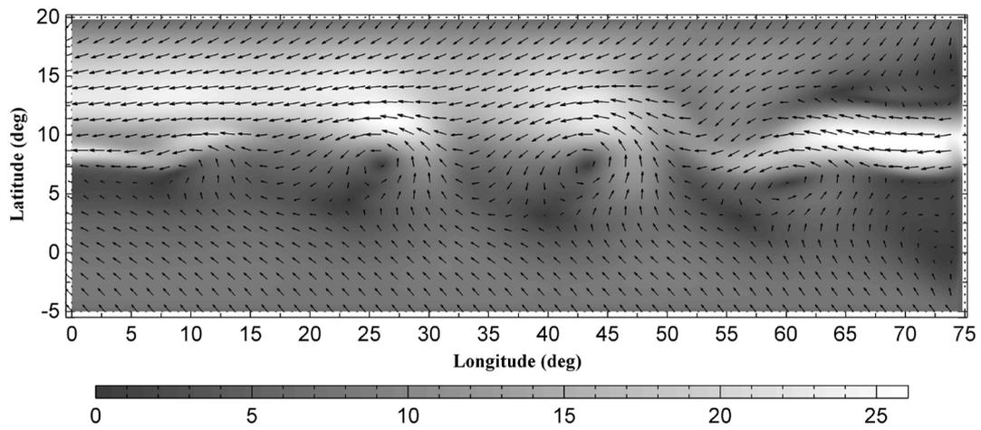
**Figure 3.** The distribution of horizontal component of the air velocity (m/s) at the altitude of 600 m, computed 50 hours after the beginning of calculations. The degree of shadowing of the figure indicates the module of the velocity in m/s.
