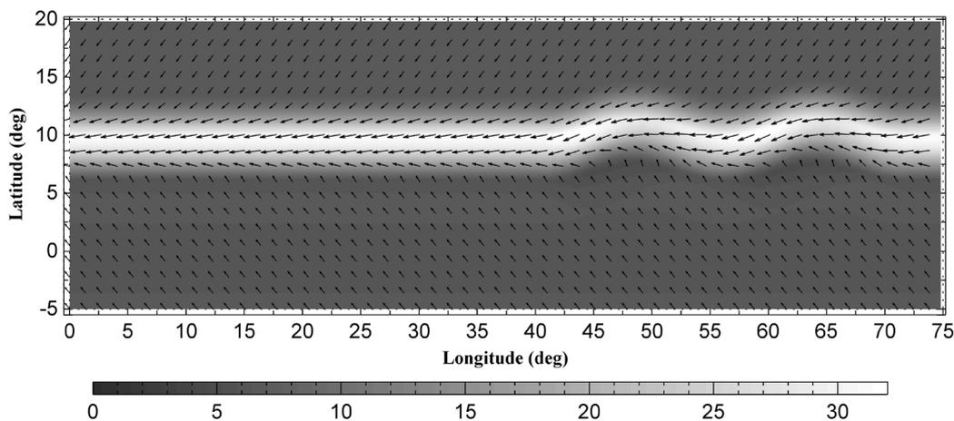
**Figure 1.** The distribution of horizontal component of the air velocity (m/s) at the altitude of 600 m, assigned at the initial moment. The degree of shadowing of the figure indicates the module of the velocity in m/s.
