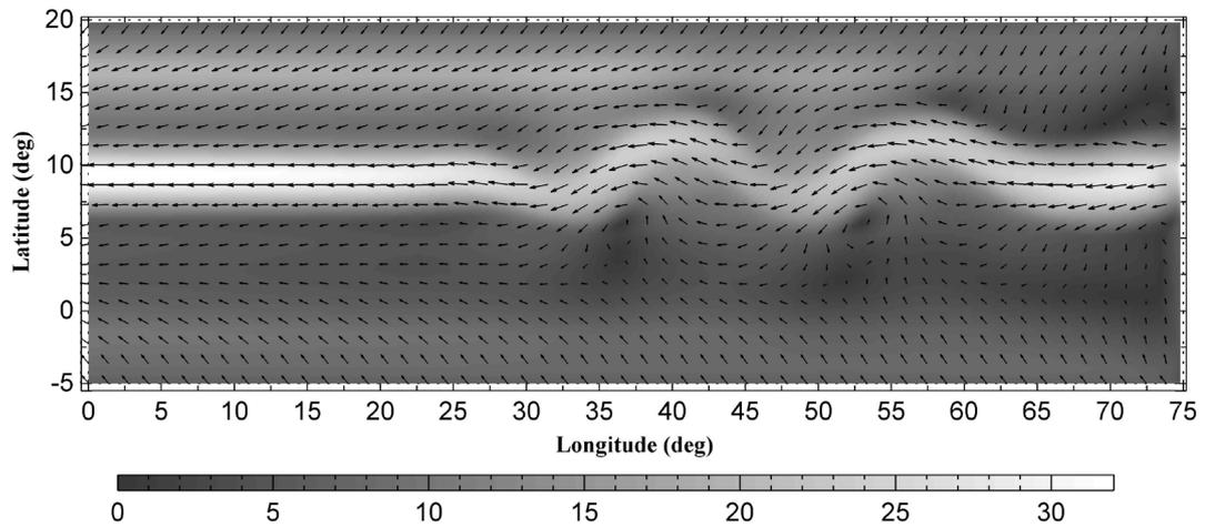
**Figure 2.** The distribution of horizontal component of the air velocity (m/s) at the altitude of 600 m, computed 20 hours after the beginning of calculations. The degree of shadowing of the figure indicates the module of the velocity in m/s.
