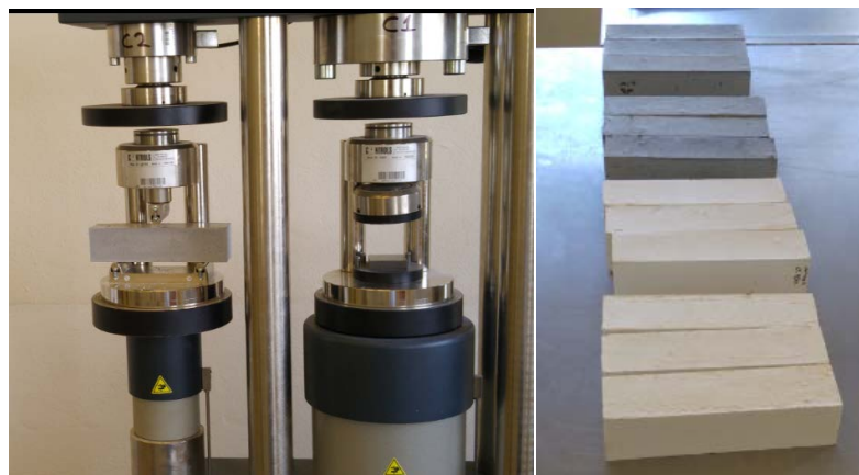
Figure 3. Bending/Compression equipment and specimens.
