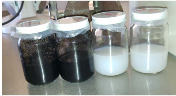
Figure 1. MWCNTs and HNTs sonicated dispersions.
