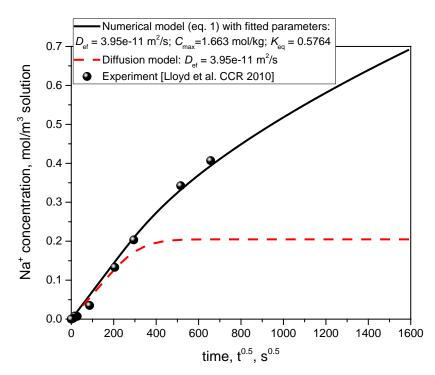
Figure 1. Comparison of modelled and experimental results [2]. Levenberg-Marquardt inverse analysis (fitted model) obtained by minimising the sum of squared residuals resulted in estimates for  $D_{ef} = 3.95 \times 10^{-11} \text{ m}^2/\text{s}$ ;  $C_{max} = 1.663 \text{ mol/kg}$ ;  $K_{eq} =$ 0.5764 m<sup>3</sup>·mol<sup>-1</sup>.
