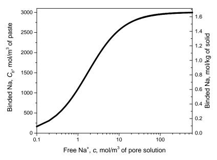
**Figure 3.** Langmuir isotherm (Equation (6);  $C_{max} = 1.663 \text{ mol/kg}$ ;  $K_{cq} = 0.5764 \text{ m}^3 \cdot \text{mol}^{-1}$ ) obtained by the inverse analysis. For better visibility logarithmic scale was used across abscissa.
