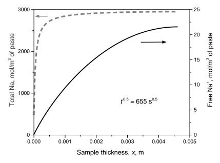
**Figure 2.** Modelled Na profile concentration across sample thickness for leaching time  $t^{0.5} = 655 \text{ s}^{0.5}$ : dashed curve for total Na showing huge values on left ordinate compared to solid curve for relatively low amount of free Na on right ordinate (same units of mol/m<sup>3</sup> of geopolymer paste).
