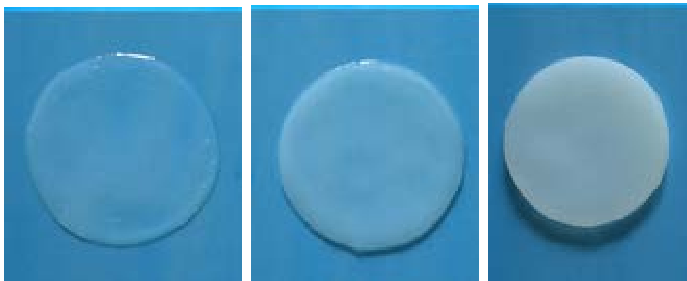
Figure 2. Bacterial cellulose 1, 7, 14 days (left to right), the thickness of bacterial cellulose depends on growth time.
